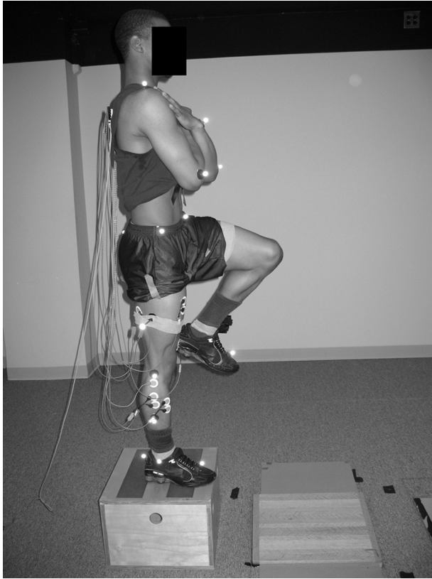
Figure 1. Laboratory setup for 30-cm drop landings. Participants crossed their arms over their chest and started each trial in a single-limb stance on the dominant leg. They then dropped off of the platform and landed on the force plate using the dominant leg.
