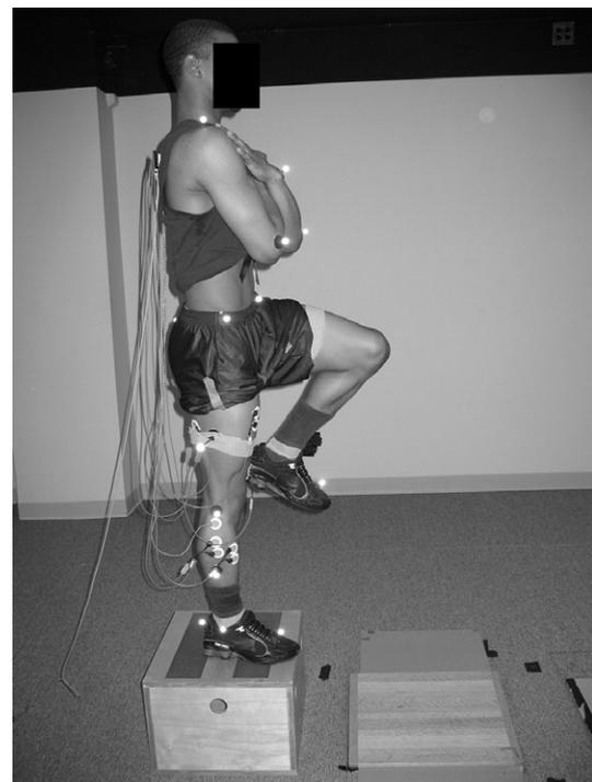
**FIGURE 1** Laboratory setup for 30-cm drop landings. Participants crossed their arms over their chest and started each trial in a single-limb stance on the dominant leg. They then dropped off the platform and landed on the force plate using the dominant leg
