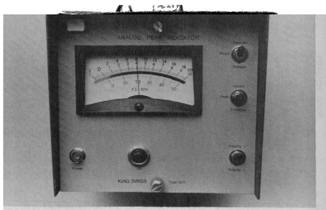
Fig. 4. Photograph showing peak analog indicator frozen at the peak value.
