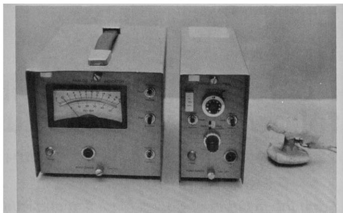
Fig. 1. Photograph of the MMTU. An electromechanical device designed by Kristal Instruments.
